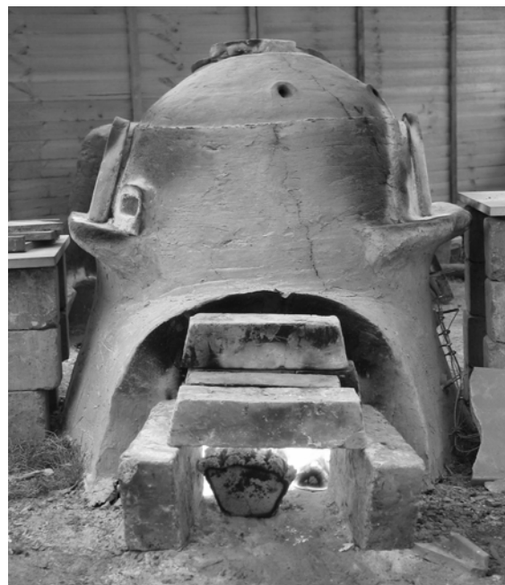
Figure 7. The rebuilt smaller furnace with gathering holes on either side, plus doors supported on shelves beneath, and the fuel chute in the foreground.
