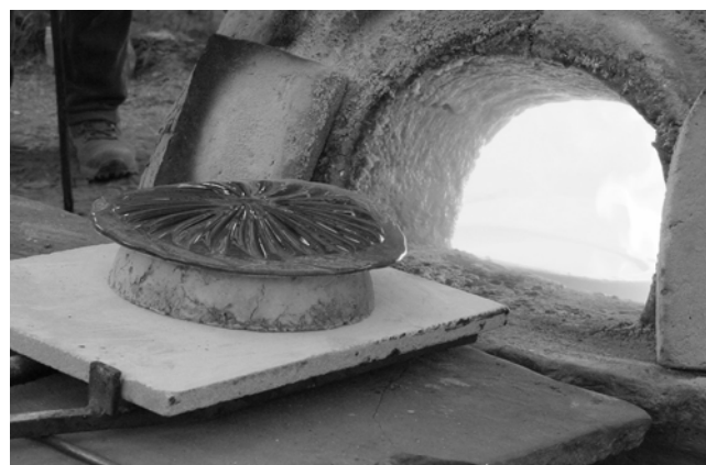
Figure 9. Ribs were pinched on the surface of a circular slab of glass, which was then laid over a dome made from daub. Together these were placed on a sandstone shelf, or bat'leth , which was slid into the furnace. The glass slumped over the dome, forming a ribbed bowl.
