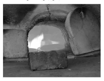
Fig. 3 View of pots in the furnace during firing (Courtesy of J. Bayley).
