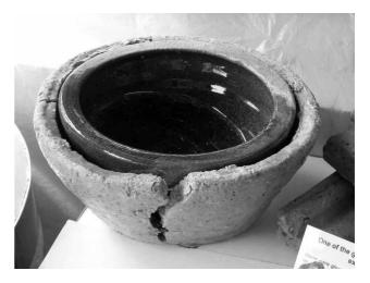
Fig. 4 A pot after firing with glassy rim (front) and deposits formed from reactions with fuel ash (back) (Courtesy of J. Bayley).
