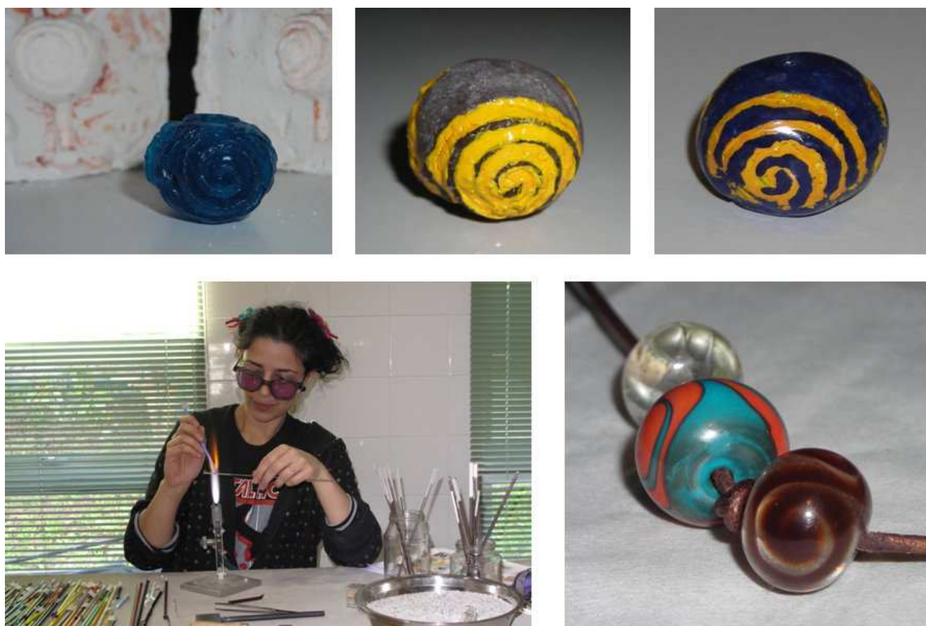
Figure 3. (Top row) three final stages in the production of moulded beads: a grooved bead just extracted from the mould and cold-worked for the removal of spruing, flashing and parting lines; the enamelling stage and a finished bead after polishing. (Bottom row) Lampworking for bead making and one of the examples of spiral beads successfully produced with this technique (©Martina Bertini).
