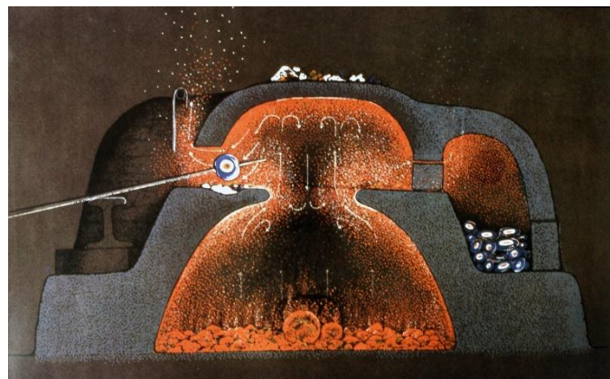
Figure 2: Diagram of historic bead furnace. © O. Küçükerman
