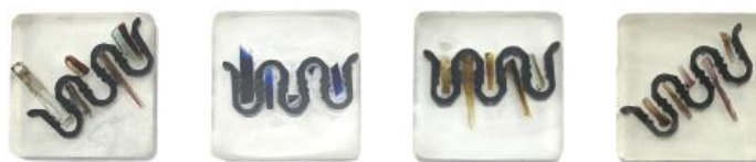
Figure 2: Samples embedded in resin blocks. Image: ©Ivona Posedi
