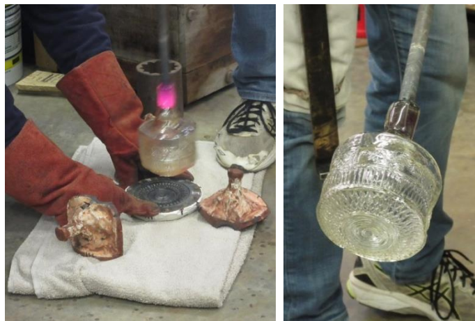
An 'Ennion cup' being taken out of a four-piece mould, during the blowing process © R. Tyson
