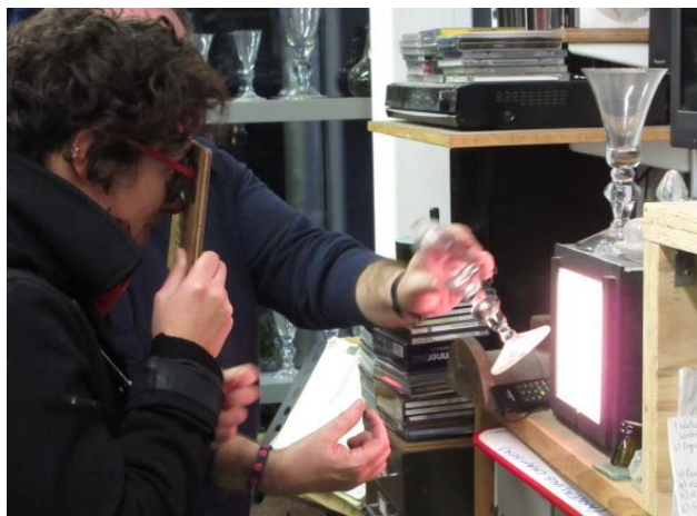
Viewing strains in unannealed glass through a cross polarising filter, against a light box © R. Tyson
