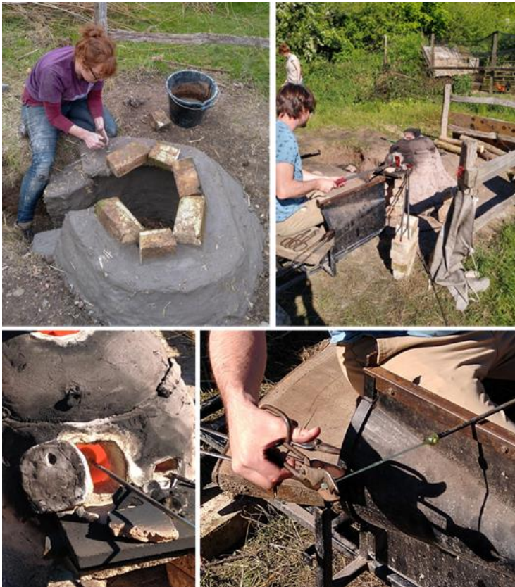
Figure 3: (top left) constructing the furnace, (top right) Colin Rennie working at the furnace during week 1 of the experiment (bottom left) the gathering hole during glassblowing being used to reheat the vessel, (bottom right) pulling a cane: the ease with, and length to which a cane could be pulled using one smooth, continuous pulling motion was used to help assess the workability of the glass. Photos © Victoria Lucas
