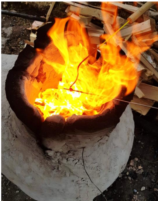
Figure 6: The making of a bead. The red-hot glass cane is wound on a mandrel. Photo © Eleonora Montanari
