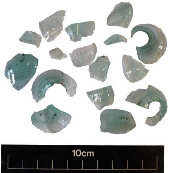
Figure 4: glass cullet and moils remaining after the fifth recycling cycle at the end of week 2. Photo © Victoria Lucas
